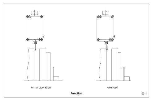
It is possible with SIKUMAT® Torque Limiters to utilise the axial movement during an overload occurrence to actuate a proximity switch so that when the preset limit torque is exceeded, the drive can be switched off electrically and/or a signal can be triggered.
